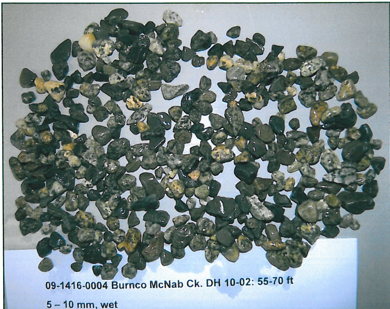
Figure 1. Photo of the passing 10 mm, retained on 5 mm sieve fraction, showing the oxidation staining on many of the granitic particles and flat and/or elongated particle shapes of some of the metamorphic rock types. Water was applied to the sample to make colour and texture more visible.
