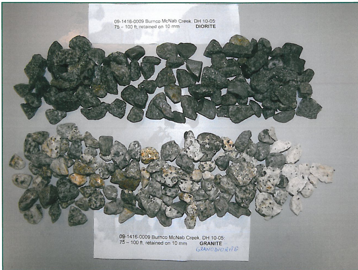
Figure 1. Granite/granodiorite and diorite particles in the retained on 10 mm portion of the sample. Water was applied to the sample to make colour and texture more visible.
