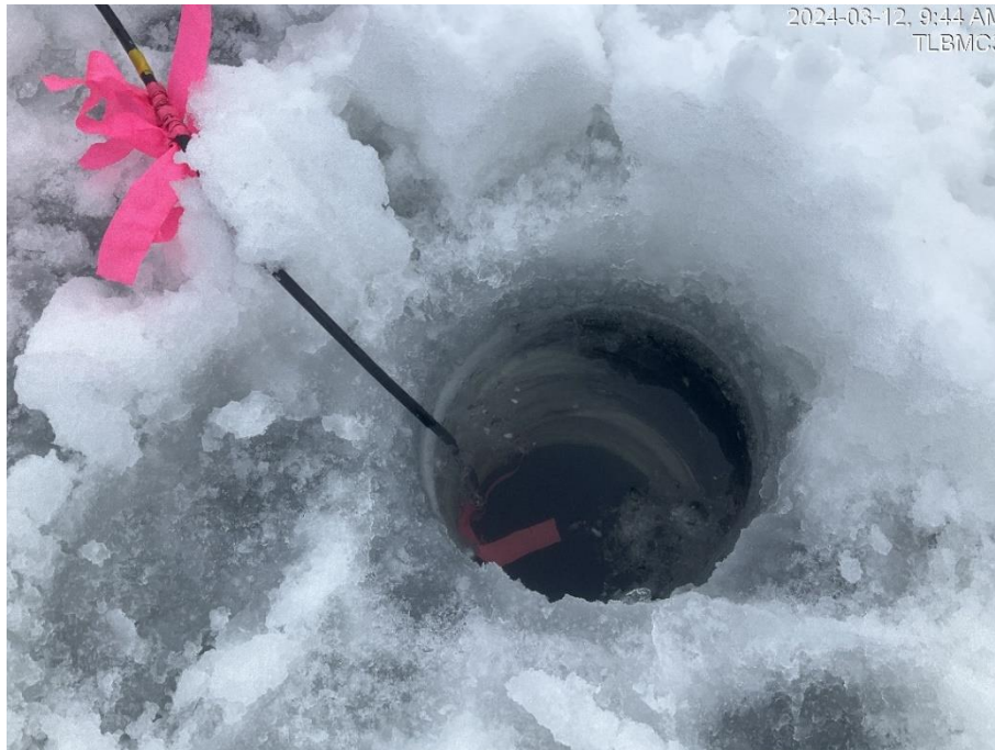
Photo 5. TL BMC3 - View of augered hole showing ice depth and condition at sampling site.
