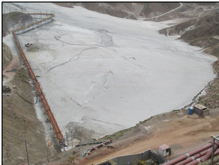
Photograph 1 – Irrigation Dust Control at Cerro Verde Mine
