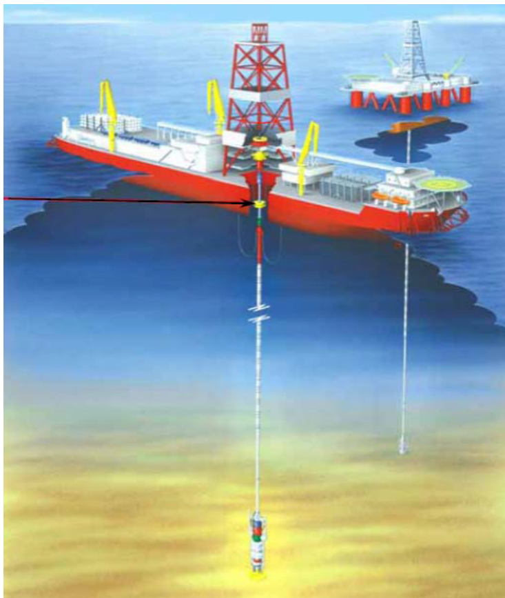
Figure 2 Illustration of Drill Ship (front) and Semi-submersible (back)
