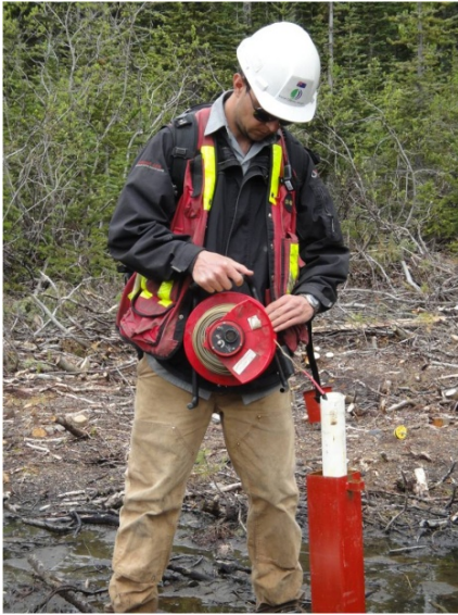
Figure 2.2 Measuring Water Level in an Open-hole Piezometer with Diptape
