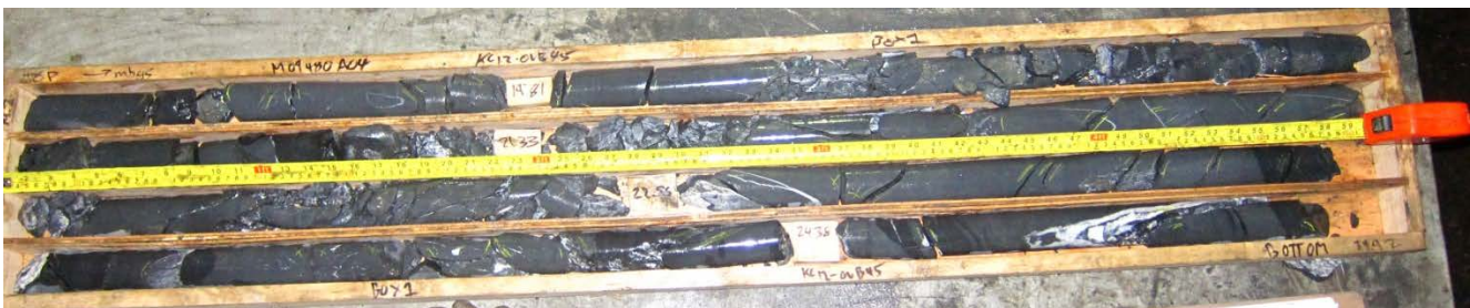
Figure 3.5 KC12-OVB45 NQ Rock Core from 18.91 m to 24.77 m
