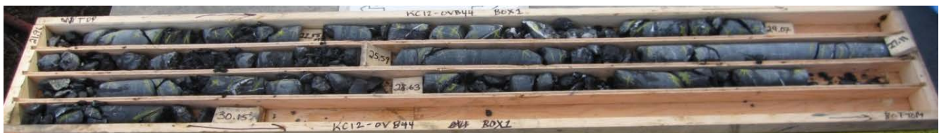
Figure 3.4 KC12-OVB44 NQ Rock Core from 21.96 m to 30.2 m
