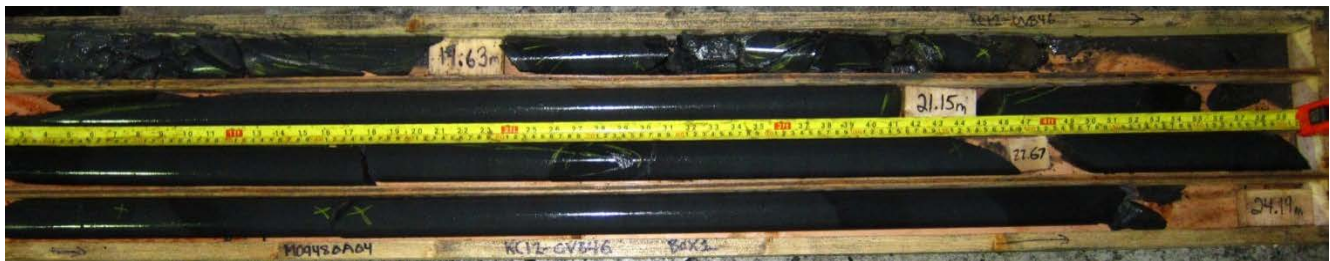
Figure 3.7 KC12-OVB46 NQ Rock Core from 18.8 m to 24.19 m
