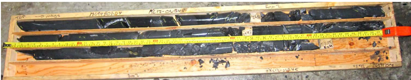
Figure 3.6 KC12-OVB45 NQ Rock Core from 24.77 m to 28.95 m
