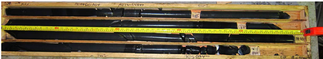
Figure 3.9 KC12-OVB47 NQ Rock Core from 10.92 m to 16.10 m
