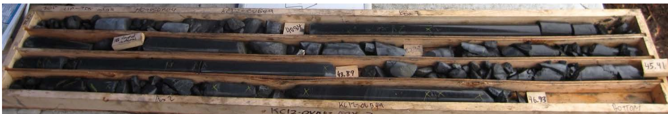
Figure 3.11 KC12-OVB49 NQ Rock Core from 39.3 m to 46.93 m
